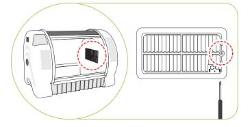
▶ Separte cover by bending Picture ⓐ, ⓑ to the left at the same time and using your fingers or a screwdriver, then pulling in the direction of Picture © and pulling to the front of direction in Picture (d). At this point do NOT completely remove the silicon hose from the cover, but follow Picture @ which will allow easier assembly (using tools will help).
