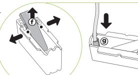
▶ Take out float ① by slightly spreading using your hand and clean the scale inside humidifying container. [Fig-3] (Clean once every week)
