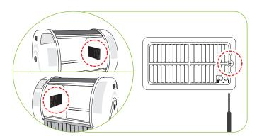
▶ Separte cover by bending Picture ⓐ, ⓑ to the left at the same time and using your fingers or a screwdriver, then pulling in the direction of Picture ⓒ and pulling to the front of direction in Picture ⓓ. At this point do NOT completely remove the silicon hose from the cover, but follow Picture ⓔ which will allow easier assembly (using tools will help).
